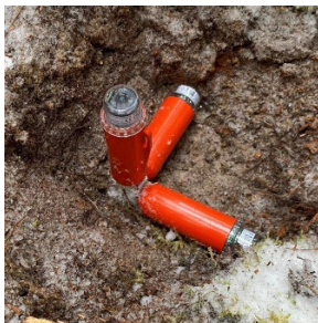
Image of the probe used to measure the soundwaves for the KRCEE seismic investigation.
